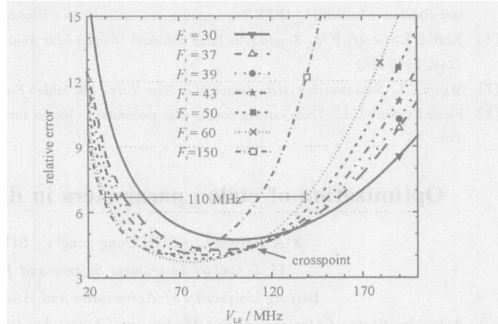
Fig. 5 Relative error vs frequency offset of laser to Fabry Perot interferometer
