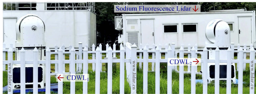
Fig. 1. Two CDWLs in front of the Na lidar, all developed by LidarX group at USTC.
